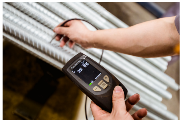
Control of coating thickness
